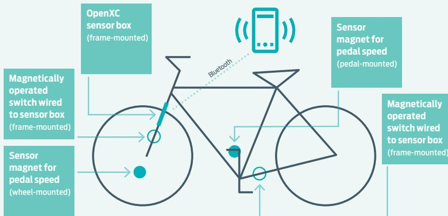
First, the electronic sensor box gathers sensor data, then the accompanying software libraries and application programming interface provide a way for developers to create custom applications and sensors.
